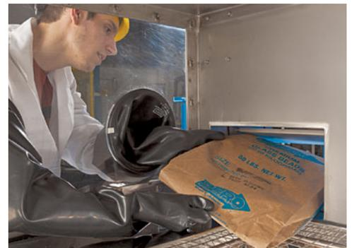
*An operator transfers empty bags from the glove box side of the enclosure through a bag infeed chute in the enclosure sidewall, drawing dust generated from bag compaction as well as dumping activities into the integral dust collection system.*
